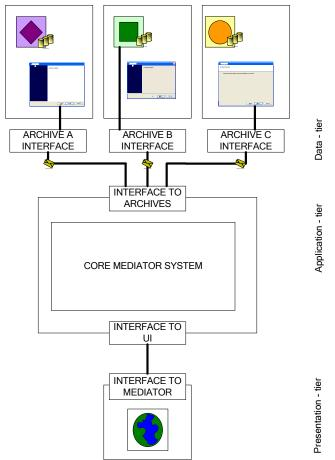
Figure 1. A typical 3-tier architecture for a multimedia mediator.
